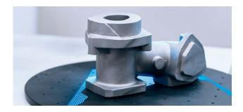
Casting & Forging – ATOS Core shortens the measuring and inspection times in sand, pressure die and investment casting as well as in the forging industry.
